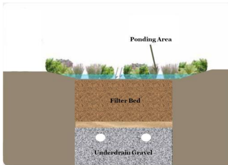
Figure 1. Bioretention Schematic (WVDEP)
