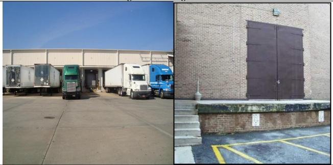
The **left panel** shows a truck loading and unloading area that is covered to prevent rainfall from washing away spilled products, whereas the **right panel** shows an uncovered loading area with a high potential for pollutant wash-off into the adjacent storm drain system
