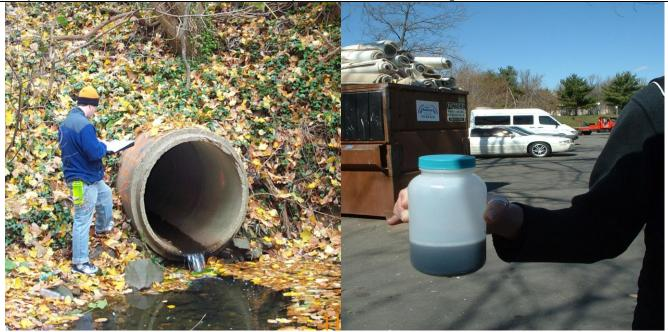
All storm drain pipes that daylight from the facility should be checked for suspicious flows during dry weather (left). Even small diameter storm drain pipes can be a source of episodic or transitory illicit discharges of pollutants (right)
