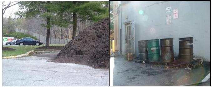
**Left panel:** When it rains next, this mulch mountain will send polluted runoff into the storm drain at far left. **Right panel:** This restaurant has poor storage of cooking grease which leaks into the storm drain system. Simple best practices can prevent materials stored outside from becoming a stormwater runoff problem
