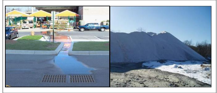
Wash-water from outdoor plant sales in this big box store is sending nutrient-rich water directly into the storm drain (left). The large pile of un-covered road salt at this facility sends a toxic pulse of high salinity water into the nearby stream during every rainfall event (right). Better storage and management of road salt can prevent this problem.
