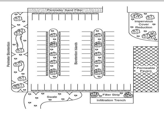
The graphic above shows the many different retrofit options available to treat the quality of stormwater runoff within or along the margins of a typical parking lot, including filter strips, swales, perimeter or island bioretention, sand filters and impervious cover reduction.
