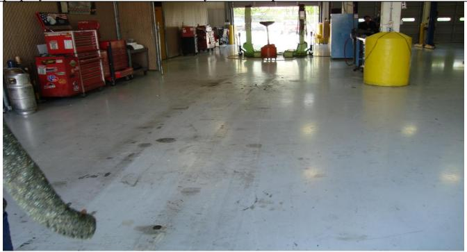
This indoor truck maintenance area keeps pollutants away from rainfall and stormwater. The shop drain is connected to the sanitary sewer system rather than the storm drain system, and has proper storage for used fluids, rags, solvents and other materials.
