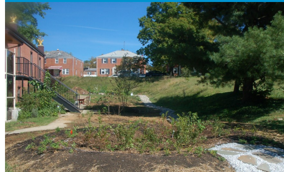
After: New rain gardens installed throughout the site capture water runoff and create a space for nature and mindfulness to grow.
